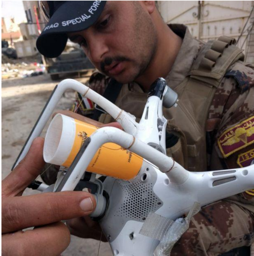
Figure 6: A UAV that carried a 40mm rifle grenade 6
